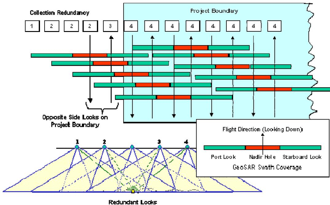
**Figure E.11. Illustration of GeoSAR’s Redundant Area Coverage**
