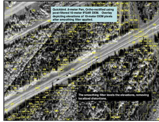
Figure 27. A smoothing filter leveled the elevations on the road, removing localized distortions.
