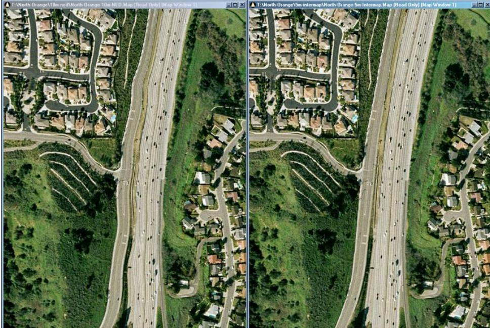
Figure 18. Orthophoto with warped roads in Orange County, CA when orthorectified w/10-meter NED DEM.
