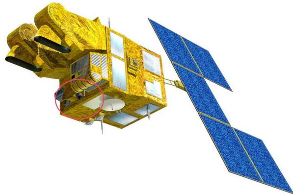
SPOT 5 satellite, red circle shows HRS secondary payload.
