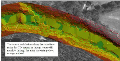
**Figure 15. DTM prior to hydro-enforcement.**
