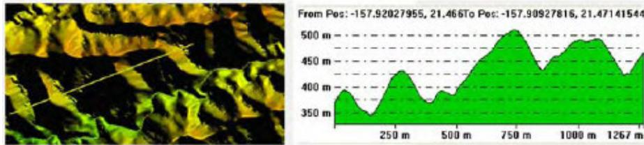
Figure E.9. A profile through the shadow regions, indicated by the yellow line in the DTM image on the left, is presented in the chart to the right to demonstrate that there is elevation data in areas of shadow regions.
