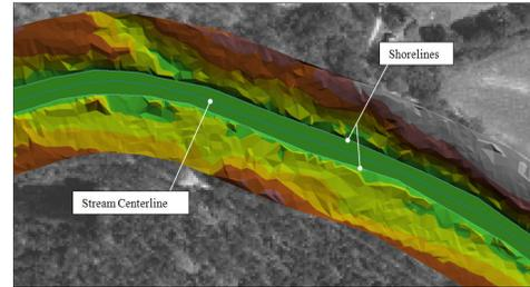
**Figure 16. DTM after hydro-enforcement**
