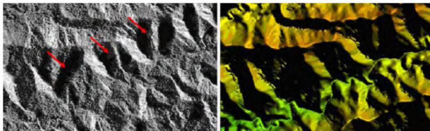
**Figure E.8. Dark region (indicated by red arrows in the ORI, left image) are regions of shadow where the radar pulse was not able to reach. The corresponding elevation data is illustrated in the right image.**
