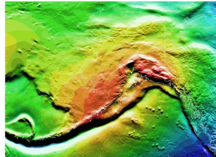
**Figure 7. The geoid model of Alaska contains vertical errors as large as 2 meters, compared with a few centimeters in the lower 48 states.**
