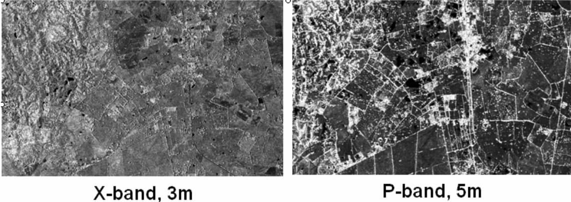
**Figure E.13. Fence lines and powerlines in X and P-band. Compared to X-band, P-band has much greater sensitivity in detecting fences and power lines.]**
