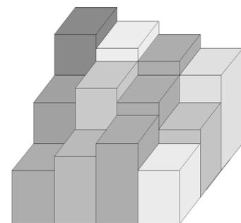
**Figure 17. DEM cells are called “voxels” (3-D or volume pixels)**
