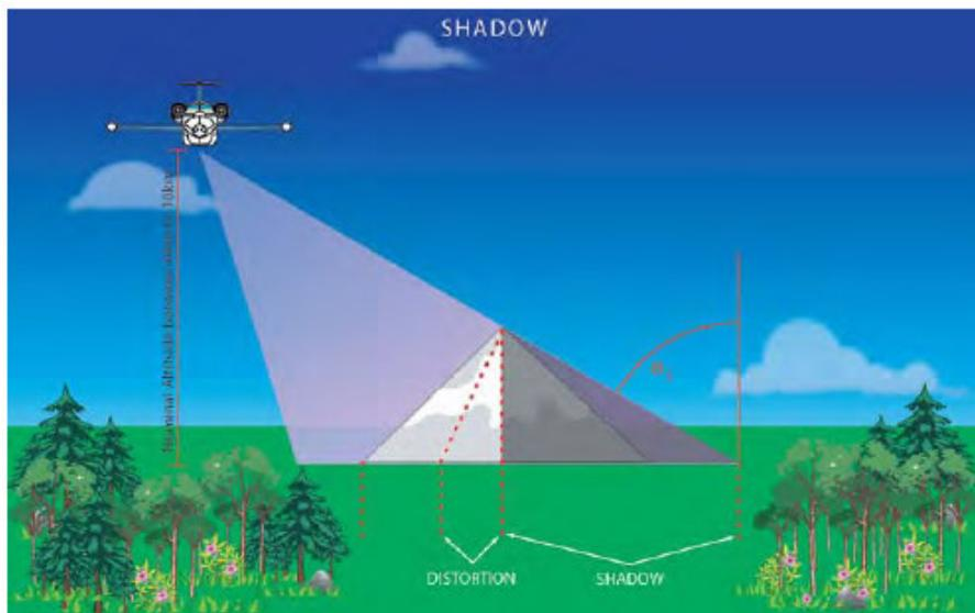
Figure E.6. Radar shadow illustrated.
