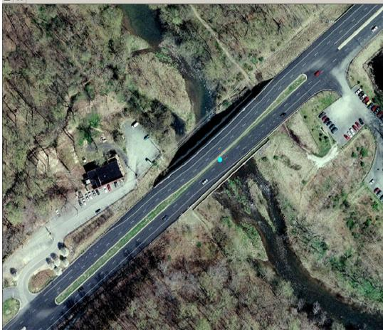
**Figure 22. Orthophoto with warped bridge due to DTM orthorectification.**
