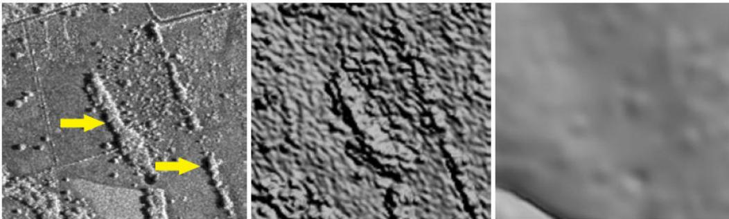
**Figure E.7. Dark regions behind trees; ORI left image, DSM middle image, DTM right image**
