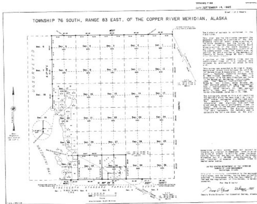
**Figure 10. The example plat shown here is of a township that contains hydrography delineated photogrammetrically. The plat notes in the margin state the following:**
