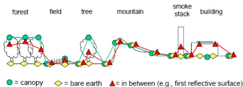
Figure 5 — In FAA and ICAO terminology, the term “terrain” could pertain to the tree canopy, bare earth, or something in between such as the first reflective surface. As used in this report, the term “DTM” refers to the bare earth elevation surface (yellow), and the term “DSM” refers to either the canopy (green) or the top (first) reflective surface (red).
