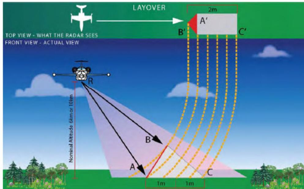
**Figure E.2. The geometry of layover. The perceived effect is that the red area is smaller than it actually is. In the top view, it appears as less than ½ meter, but in the front view, you can see that the red area actually covers more than ½ meter.**
