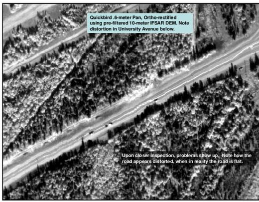
**Figure 24. Orthophoto with warped road when image is orthorectified to 10-meter IFSAR DSM.**
