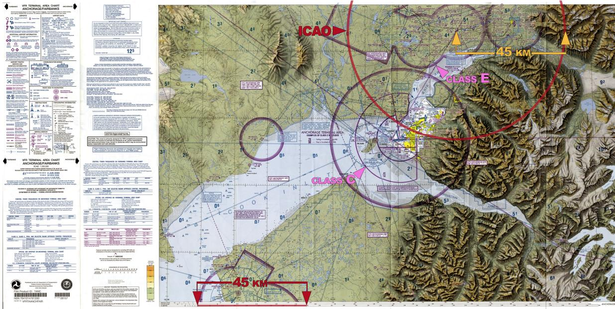
Figure B.8. VFR Terminal Area Chart showing red circle within which elevation data with 20-ft contour accuracy would be required when landing under IFR conditions at the Wasilla, Alaska airport.
