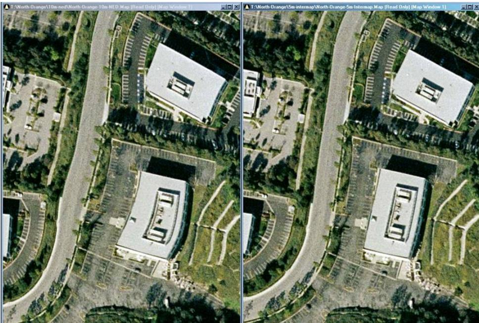
Figure 20. Orthophoto with warped building in Orange County, CA when orthorectified w/10-meter NED DEM.
