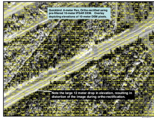
**Figure 25. Grid elevations shows the road is warped due to variable elevations of grid cells on the road.**
