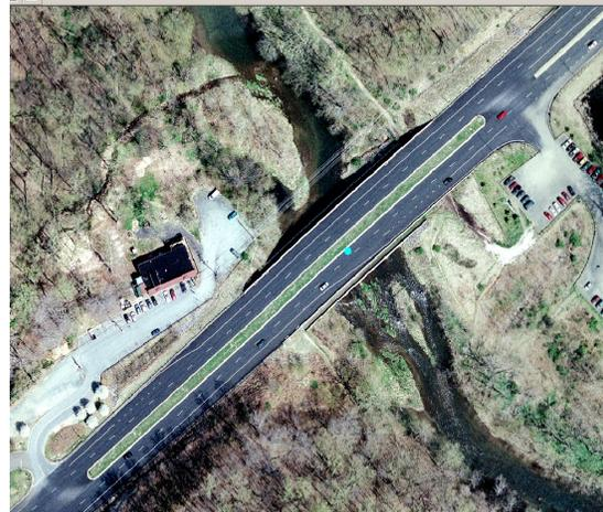
**Figure 23. Orthophoto with correct bridge due to DSM orthorectification.**
