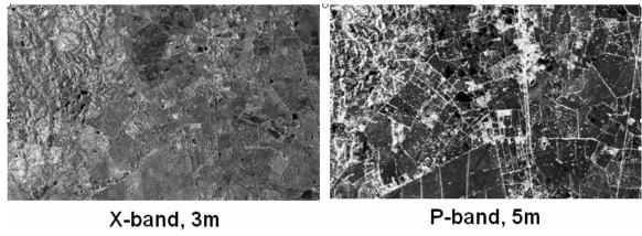
Figure E.13. Fence lines and powerlines in X and P-band. Compared to X-band, P-band has much greater sensitivity in detecting fences and power lines.]
