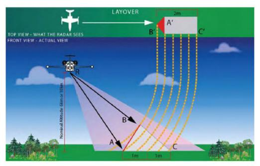
Figure E.2. The geometry of layover. The perceived effect is that the red area is smaller than it actually is. In the top view, it appears as less than ½ meter, but in the front view, you can see that the red area actually covers more than ½ meter.
