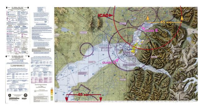
Figure B.8. VFR Terminal Area Chart showing red circle within which elevation data with 20-ft contour accuracy would be required when landing under IFR conditions at the Wasilla, Alaska airport.
