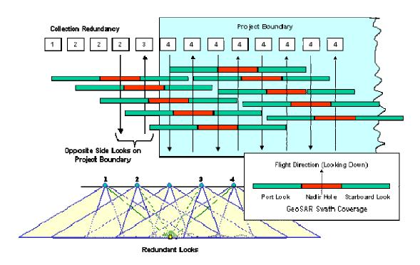
Figure E.11. Illustration of GeoSAR's Redundant Area Coverage
