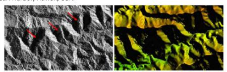
Figure E.8. Dark region (indicated by red arrows in the ORI, left image) are regions of shadow where the radar pulse was not able to reach. The corresponding elevation data is illustrated in the right image.
