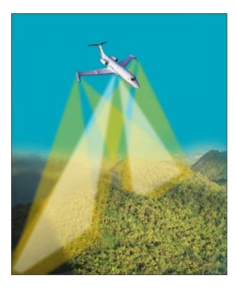
Figure E.10. Dual-sided configuration of the GeoSAR
