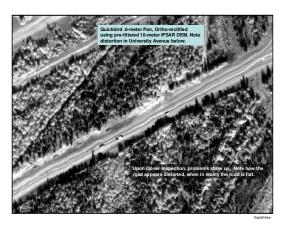
Figure 24. Orthophoto with warped road when image is orthorectified to 10-meter IFSAR DSM.
