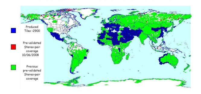
This graphic shows Reference3D product status as of June 30, 2008. 2,900 one degree geocells (blue tile area) have been produced. The green and red areas show validated HRS stereo pair coverage, over 122 M KM2 globally.
