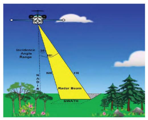
Figure E.1. Radar sensor geometry example of our system configuration in which the radar beam (in yellow) has an incidence angle range from 35° to 55°. The location of the near range (NR) and far range (FR) and swath width are also indicated. At a flying height of 10.4 km (34,000 feet), our swath width is approximately 11.5 km in width. A typical flight line can be as long as 1200 km
