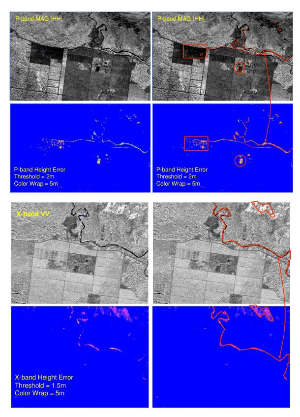
Figure E.12. Height Error Example Agricultural Field (P-band/X-band, 5m Post)
