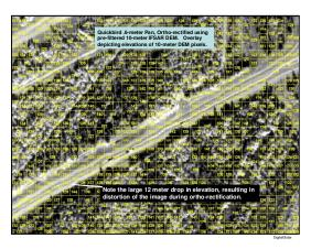
Figure 25. Grid elevations shows the road is warped due to variable elevations of grid cells on the road.
